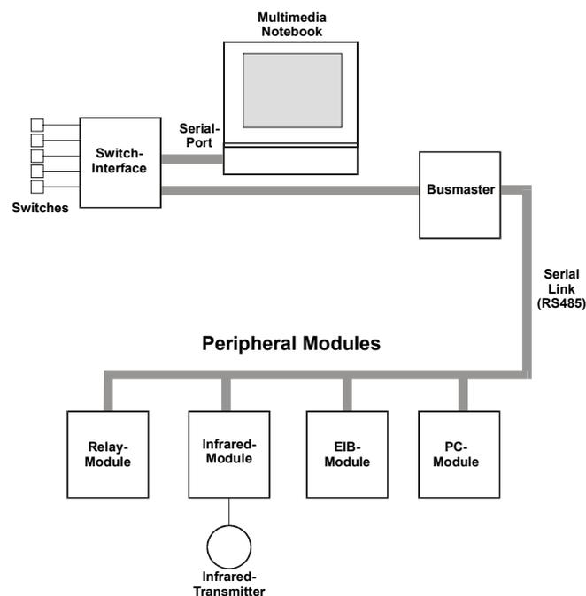
Fig. 5: Structure of Autonomy prototype system used at smart room at Elisabethinum. Twisted Pair EIB is connected via RS-232 link to EIB-Module which itself is part of a RS-485 based Autonomy field bus system.
