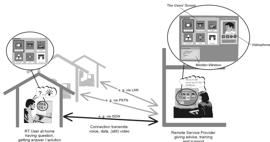
Fig. 6: Remote service provision for PC based RT systems designed by EU funded RESORT project.
