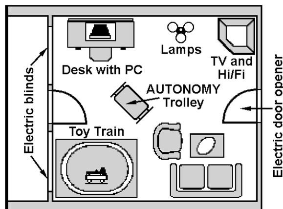
Fig. 3: Smart Room at support centre Elisabethinum in Axams near Innsbruck. Equipped with EIB Twisted Pair and the AUTONOMY system in 1995.
