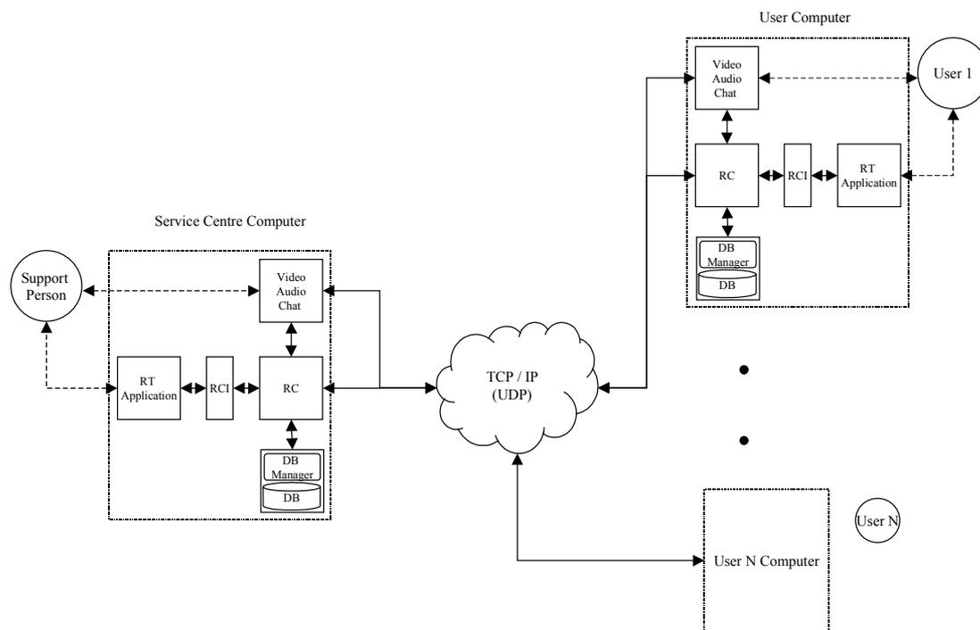
Fig. 7: RESORT system structure: On the left hand side the RESORT Service Centre, on the right hand side the RESORT Client PCs (at special schools, residential areas or private home). In between the Network.
