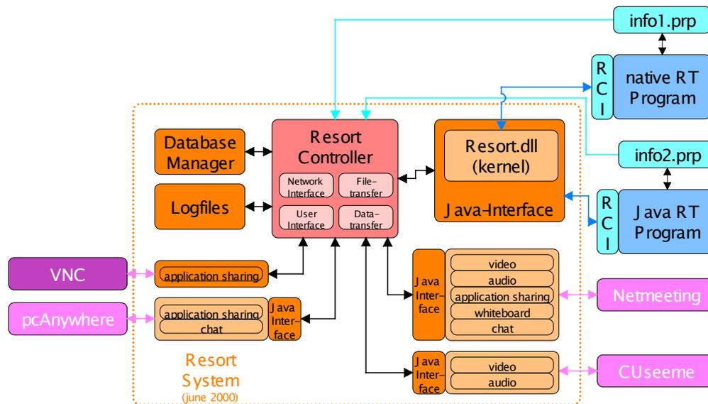
Fig. 8: Modules and interfaces of the RESORT prototype system. Different available third party products for audio, video and data conferencing can be used. The current prototype uses H.323 and T.120 implemented by Microsoft Net-meeting v3 product. For RCI specification refer to [12,22].
