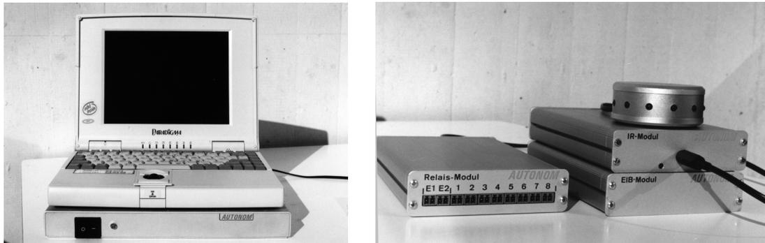
Fig. 4: Autonomy user interface implemented on MS Windows based laptop, below Busmaster of Autonomy fieldbus system (left picture). Three peripheral modules for input/output, infrared and EIB-Link (right picture).
