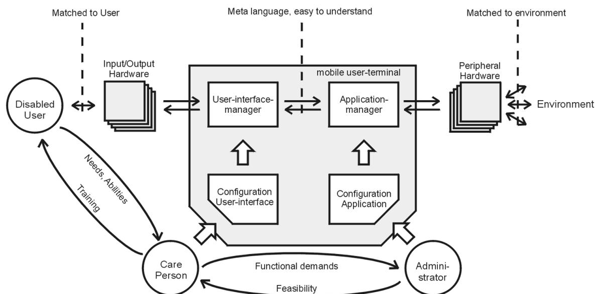
Fig. 1: Block diagram of the AUTONOMY system showing interaction between system components and user groups [5,6,7].
