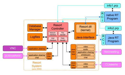
Figure 3: Modules and Interfaces of the RESORT prototype system. Different available third party products for audio, video and data conferencing can be used. The current prototype uses H.323 and T.120 implemented by Microsoft Netmeeting v3 product. For RCI specification refer to [5].
