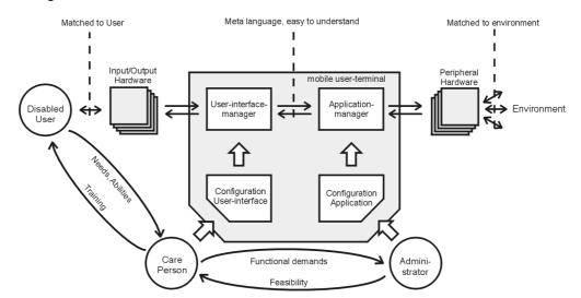
Figure 1: Block diagram of AUTONOMY system showing interaction between system components and user groups
