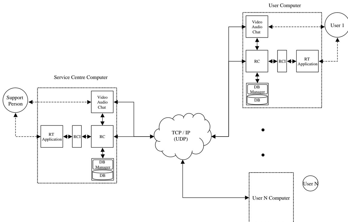
**Figure 2. Overview of RESORT system structure: On the left hand side the RESORT Service Centre, on the right hand the RESORT Client PCs (at special schools, at residential areas, private home, ...). In between the Network (LAN, ISDN, cable,...).**
